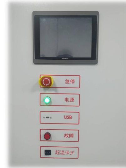
Cabinet control panel (emergency stop switch, over- temperature protection, communication interface, etc.)
