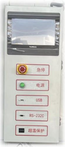
Cabinet control panel (emergency stop switch, over-temperature protection, RS-232 communication interface)
